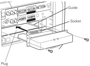
Figure shows HD DATA WIRELESS Receiver Board
